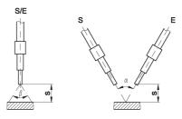
The angle " $\beta$ " with approx. 67° results of the emitting and/or the reception angle of the glass fiber.  $\beta$  is a constant and not depending on the active diameter of the glass fiber or the sensing head design. The sensing range "s" depends on the glass fiber diameter, the reflectivity (surface condition of the object as well as the angle " $\alpha$ ".
