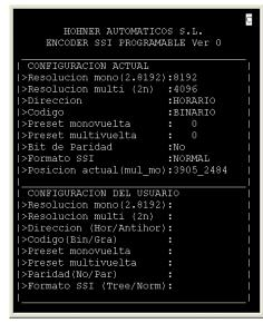
Once we have entered all the parameters, the encoder will be programmed and the screen will refresh updating the ENCODER CONFIGURATION.
