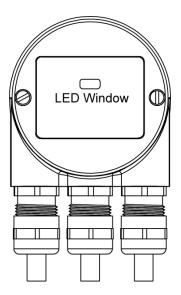
Two LEDs are implemented in the connection cap. They optically indicate the status of the encoder in the Profibus network.
